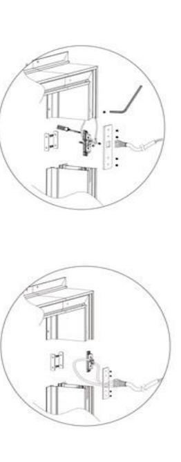
1 Remove the wire of TS-P2 power connector which on the end of TS-R90, TS-S90 corner connector
